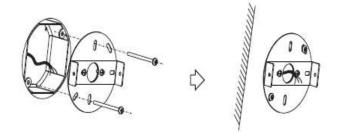
Connect wires of power supply to wires of the fixture. And fasten ground wire to green wire.
