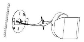
5. Mount the fixture over the backplate with 2 screws beside.
