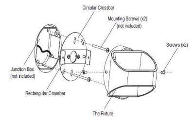
Install backplate to junction box with two mounting screws preassembled on box.Make sure wires of junction box runs through the middle hole of the backplate.
