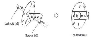
5. Mount the fixture over the backplate with 2 screws beside.
