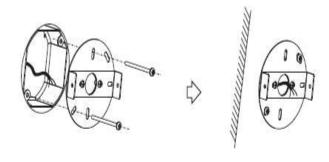
Connect wires of power supply to wires of the fixture. And fasten ground wire to green wire.
